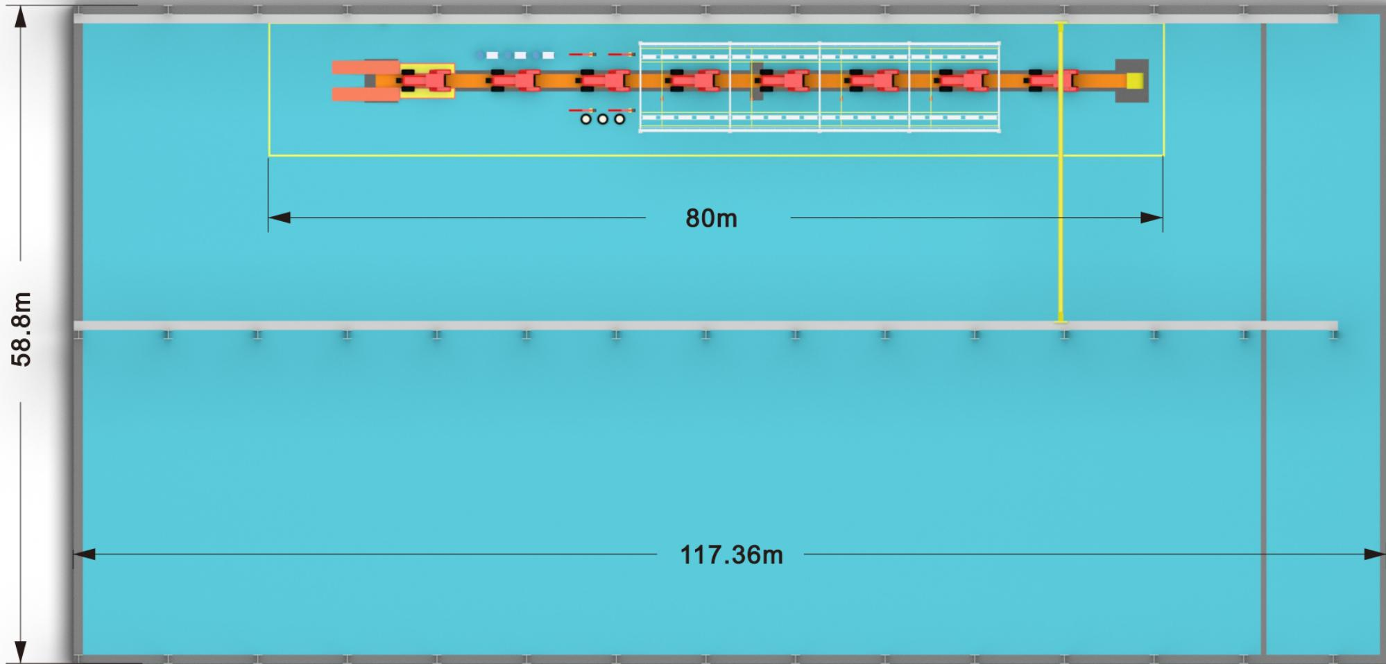
The total length of the assembly line is approximately 75 meters and it is divided into 8 assembly stations.
