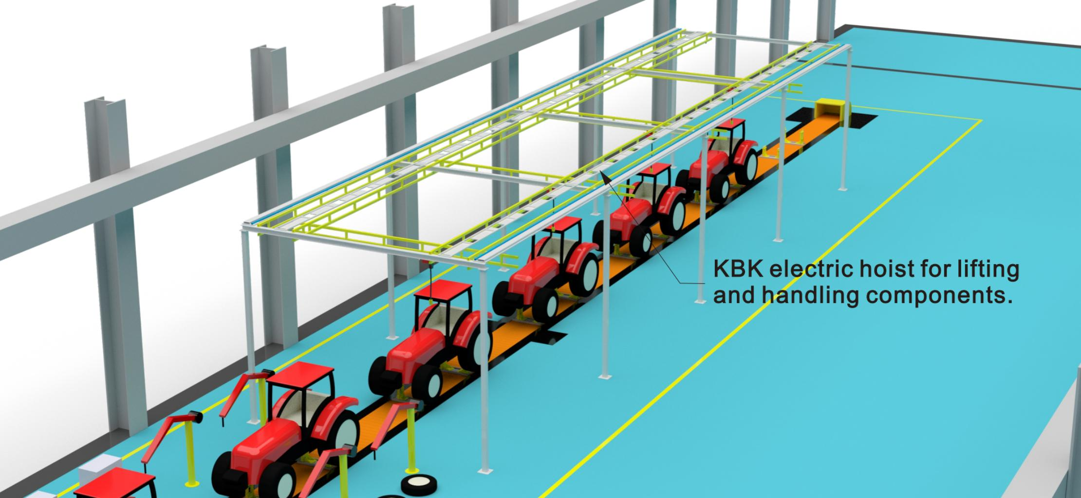
KBK electric hoist for lifting
