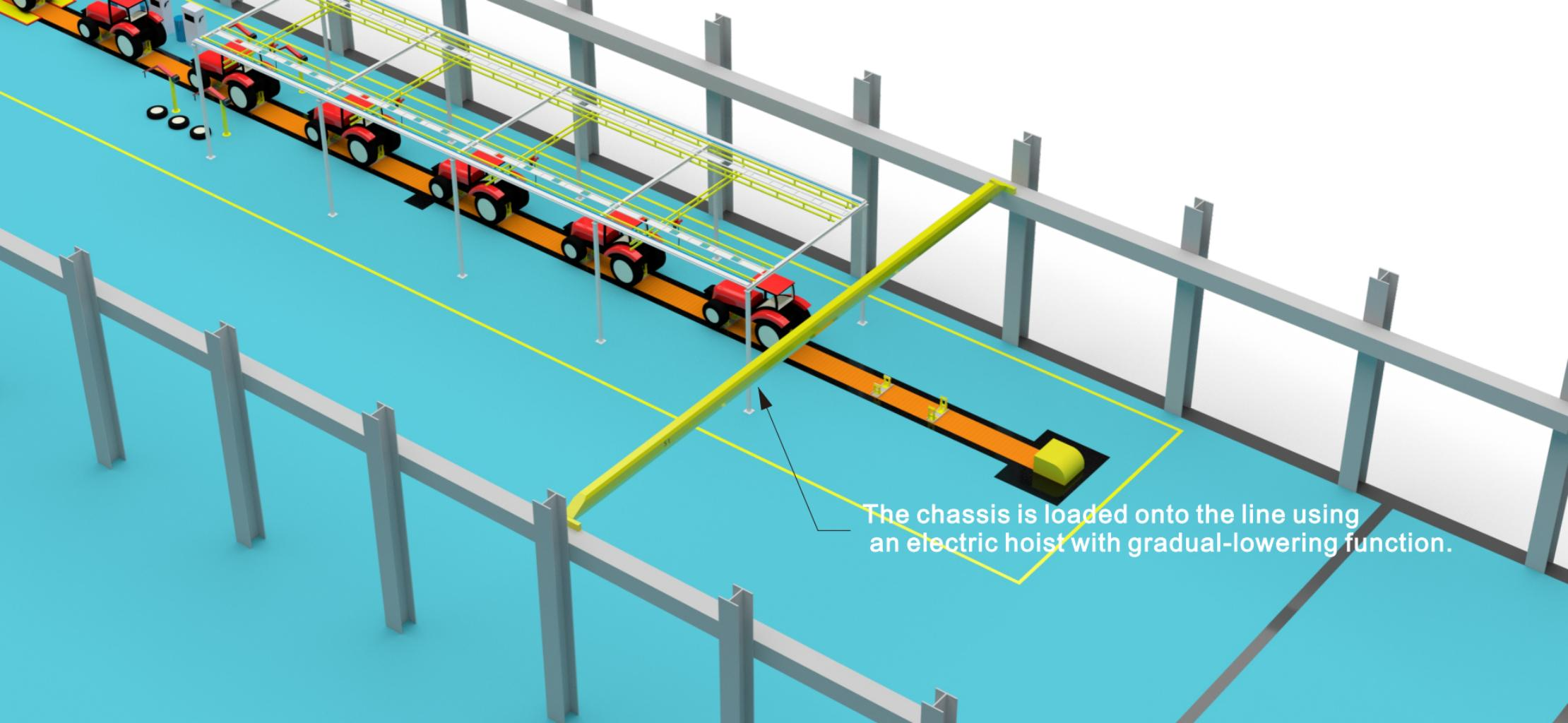
The chassis is loaded onto the line using an electric hoist with gradual-lowering function.
